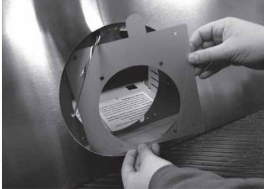
1. Remove internal blower flange plate.
