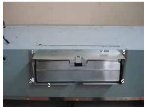
2. Secure 3-1/4" x 10" rectangular collar to back of hood using (6) M4 x 6 screws.
