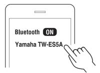
If successfully connected, you will hear the "Pairing Successful" and "Connected" audio messages in the earbud that is flashing red and blue. The indicator displays as shown below.
