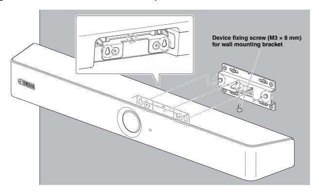
$\bf 3.$  From the underside of the wall mounting bracket, secure the device by using the included device fixing screw (M3  $\times$  8 mm) for wall mounting bracket.
