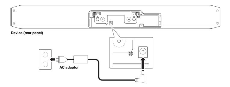
Connecting the AC adaptor automatically turns on the device.
