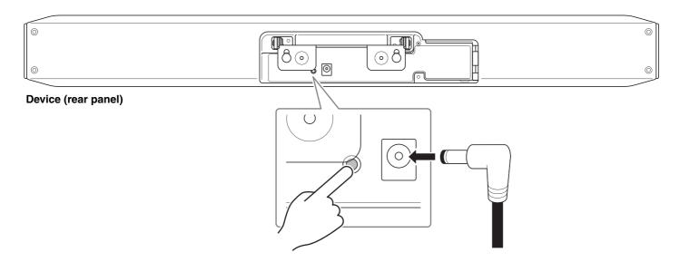
Connecting the power cable automatically turns on the device.
