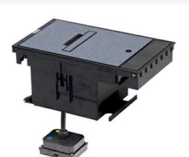
The gray Outdoor Ground Box cover assembly is prewired with (1) 30A L6-30R 240V corrosion-resistant receptacles. CAUTION: All ground box electrical circuits must be protected by a Ground Fault Circuit Interrupter upstream from the ground box.NOTE: Cover must be closed while in use. Use only molded plug and cord assemblies that are rated for outdoor use.NOTE: Maximum length of plug allowed at end of cord is 3" (76mm).
