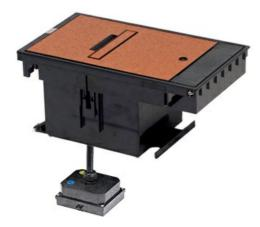
The brown Outdoor Ground Box cover assembly is prewired with (1) 30A L5-30R 120V corrosion-resistant duplex receptacles. CAUTION: All ground box electrical circuits must be protected by a Ground Fault Circuit Interrupter upstream from the ground box.NOTE: Cover must be closed while in use. Use only molded plug and cord assemblies that are rated for outdoor use.NOTE: Maximum length of plug allowed at end of cord is 3'' (76mm).
