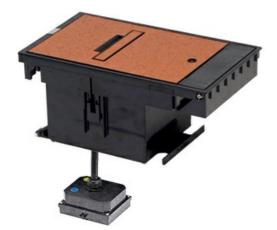
The brown Outdoor Ground Box cover assembly is prewired on a single circuit with (2) 20A weather resistant duplex receptacles. CAUTION: All ground box electrical circuits must be protected by a Ground Fault Circuit Interrupter upstream from the ground box.NOTE: Cover must be closed while in use. Use only molded plug and cord assemblies that are rated for outdoor use.NOTE: Maximum length of plug allowed at end of cord is 3'' (76mm).
