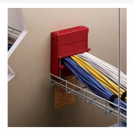
Kit includes 4" trade size split conduit sleeve to enclose existing cables, and 12" x 12" ( $305 \text{mm} \times 305 \text{mm}$ ) ceramic heat protected wall plate to cover irregular hole cuts. For use with FS4R Series Firestop.
