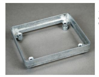
1"" (25mm) high extension. Used to increase height of preset or afterset. Die cast construction. Attach to preset or afterset with push on metal sleeves (included). Can be stacked.
