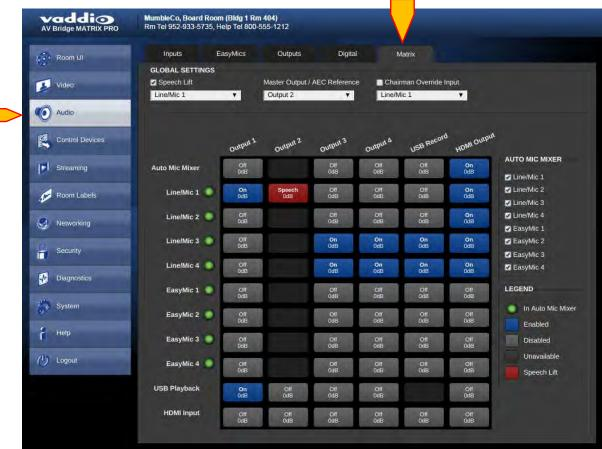
① Global Setting: Speech Lift: check to enable. Select input desired for speech lift to increase the gain through the Master audio outputs. Only one channel of Mic/Line source is available for this feature.
