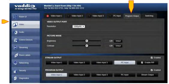
Video Output Port: Resolution pull-down allows for setting the program output resolution. This affects both the Program HDMI output and the HSDS output. Available Program output resolutions options are 1080p/60, 1080p/50, 720p/60 and 720p/50.
