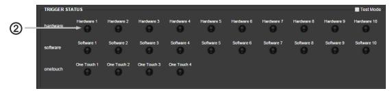
2 Trigger Button labeling: Right clicking on a trigger light button will allow you to change the label of that trigger.
