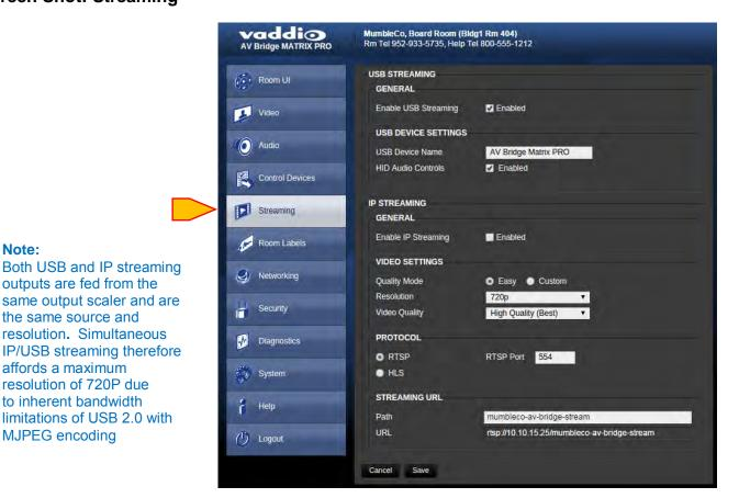
IP Streaming Settings: Streaming URL is the Network source addressing of the IP streamed output. The MATRIX PRO can support up to 4 simultaneous IP streams, all from the same URL address.
