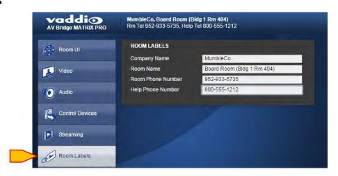
**Room Labels:** The Room Labels section provides the ability to customize room identification for remote monitoring, configuration, or control purposes. This is convenient for potentially confusing situations such as educational facilities, where many different MATRIX PRO systems may be deployed. Labeling can include Company Name, Room Name, Room Phone Number and the option for a Help line phone number.
