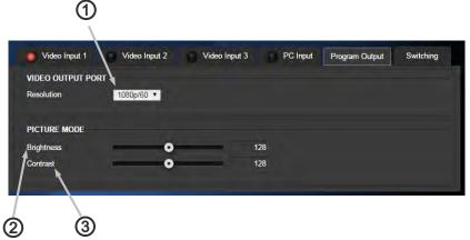
Picture Mode: Brightness control affects the Program outputs, and allows for brightness adjustment to compensate for downstream monitor displays or other destinations which lack adjustment abilities. Available adjustment range is 0-255, the numeric value is shown to the right of the slider. Once highlighted or clicked, small adjustments can be made with the arrow keys on your computer.
