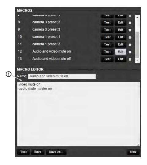
**Example Macro:** Using the Telnet commands from the CLISH list in Appendix 4, construct the Macros with the functions desired. A carriage return (keyboard Enter key) is required at the end of each command for clarity while editing and viewing. Once saved, Macros will populate the Macro list immediately above the Macro Editor, and are available for testing, trigger assignment and editing.
