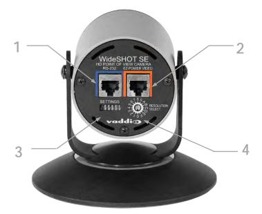
1) RS-232 Port: The RS-232 accepts modified VISCA protocol for camera control.
