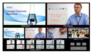
Multi-View Four-Input Layout Display for \*TeleTouch Touch Screen Control Panel (Simulated Multiviewer Output)
