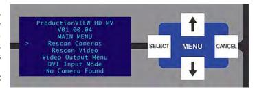
Press the arrow down button to the appropriate resolution that is compatible with your video monitor and press the SELECT Button. Press the CANCEL Button to exit out to the previous menu.
