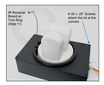
**Step 10:** Carefully put the camera assembly on top of the ceiling tile support brace, and slip the camera head through the opening in the installed tile support brace and the ceiling tile (see Step 4).
