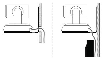
3. Attach the camera to the mount using the mounting screw supplied with the camera.
