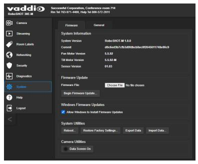
By default, the camera is set to update automatically via Windows. For this to happen, the camera must remain connected to the Microsoft Teams Rooms collaboration computer.
