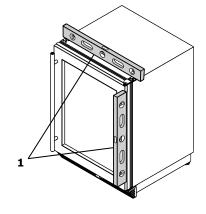
2. If the unit is not level, adjust the feet on the corners of the unit as necessary.
