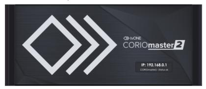
The front panel of your CORIOmaster2 includes a customizable status screen. The status screen can show the IP address of your CORIOmaster2, its status, and the name of the server.
