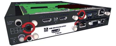
3. Grip the silver handles and pull the module forward a short distance, out of the dock on the back plane. Lift the module out of your CORIOmaster micro. Keep the module flat.
