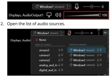
3. Select each source in turn and check the input audio level.
