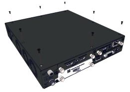
2. Remove the screws of the module or modules you want to replace. Loosen the screws of the module below the module that you want to replace.
