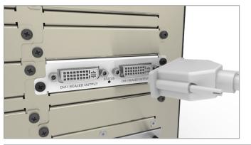
• It is recommended to use a cable mount to reduce the stress on the connector caused by heavy cables. See the installation instructions that came with your module or device.
