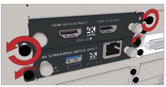
2. Loosen the screws of the module above or below the module that you want to replace.
