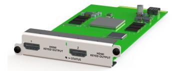
The module uses a luminance keyer. Each output has two layers, a background layer, and a foreground/keying layer. Video in the foreground layer can be keyed through from the background layer in real time with no additional latency.
