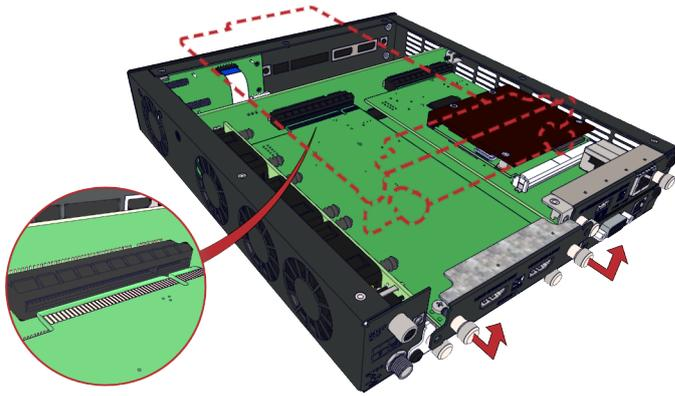
Modules with four or more inputs or outputs can be difficult to remove by hand. Some modules are designed with one or two small notches. Use the extractor tool that came with your module to hook into the notches and pull out the module.
