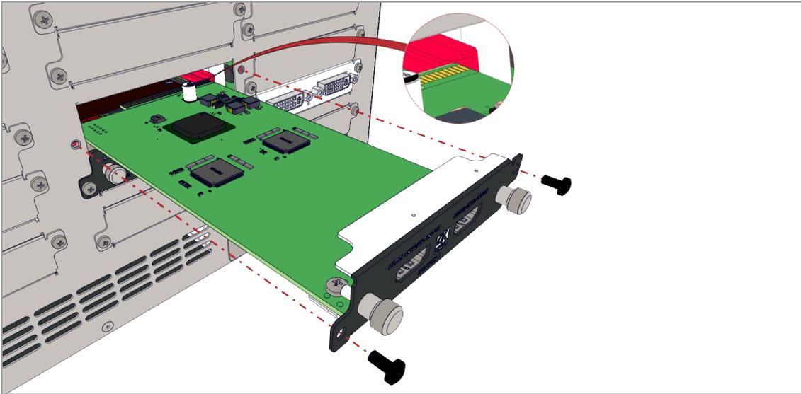
1. Insert the module into the guide rails of your CORIOmaster.
