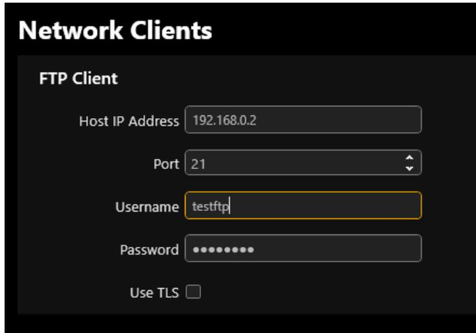
The screenshot shows the 'Network Clients' configuration interface. Under the 'FTP Client' section, there are four input fields: 'Host IP Address' with the value '192.168.0.2', 'Port' with a dropdown menu set to '21', 'Username' with the text 'testftp', and 'Password' with a masked field of seven dots. At the bottom, there is a checkbox labeled 'Use TLS' which is currently unchecked.
