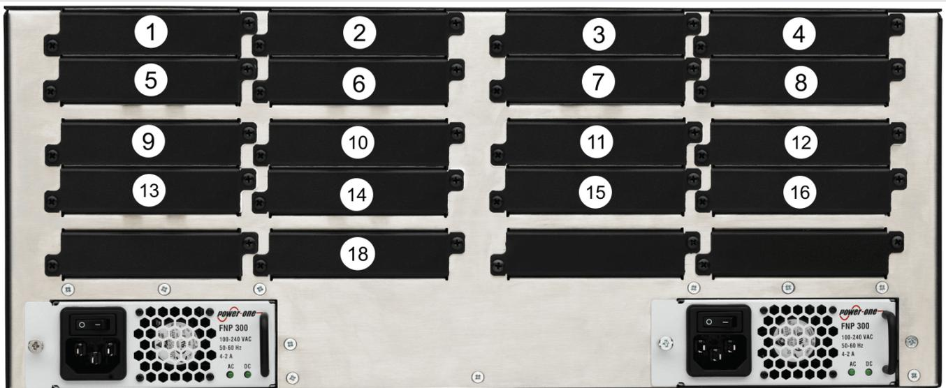
Your CORIOmaster has 16 slots that can contain input or output modules. You can have up to 14 input modules and up to 14 output modules. Of the 14 input modules, up to five can be Streaming media and 4K playback input modules. You can only have one S/DPDIF and analog audio module.
