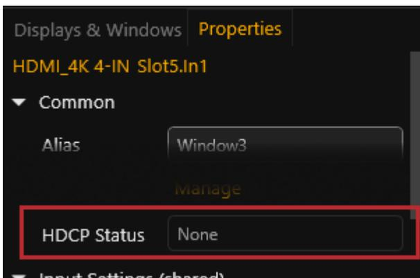
3. If you do not require HDCP you can disable it by clearing the HDCP Enabled option, or if available, select the HDCP Version which will force the input to try to negotiate that version with the source.
