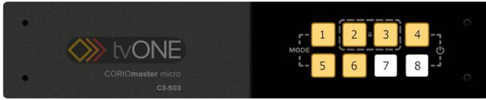
When your CORIOmaster micro is in preset selection mode, the buttons are orange. Any buttons that do not have a corresponding preset are unlit.
