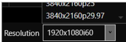
The Streaming media and 4K playback input module supports two simultaneous channels playing media. The two channels can have different resolutions, and you can choose a custom value for channel one (slot  $n$  position 1). Channel two (slot  $n$  position 2) only supports 1920x1080p60.
