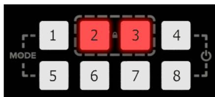
Buttons 2 and 3 are lit red The buttons of the CORIOmaster micro are locked.
