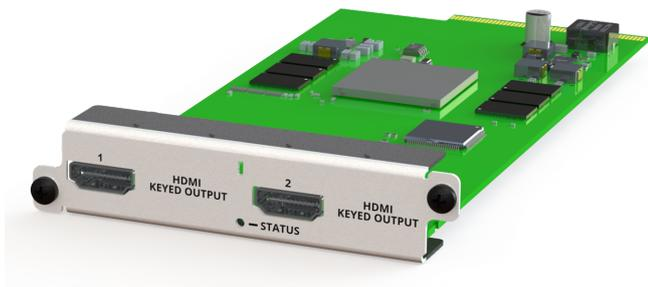
The module uses a luminance keyer. Each output has two layers, a background layer, and a foreground/keying layer. Video in the foreground layer can be keyed through from the background layer in real time with no additional latency.
