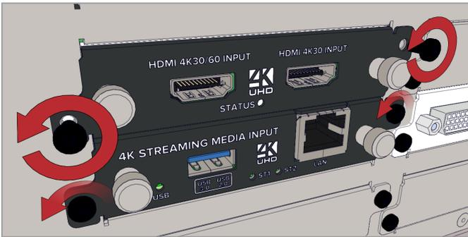
2. Loosen the screws of the module above or below the module that you want to replace.
