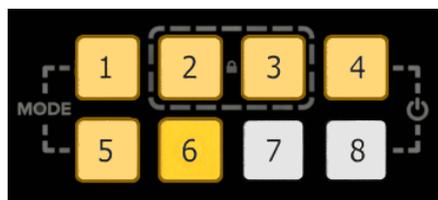
Buttons are lit dimly orange The CORIOmaster micro is in preset selection mode.
