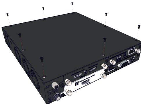
2. Remove the screws of the module or modules you want to replace. Loosen the screws of the module below the module that you want to replace.
