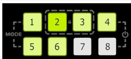
Buttons are lit dimly green The CORIOmaster micro is in source selection mode.
