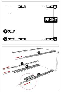
4. Use the remaining 12 M4 screws to connect the other side panel to the mounting rails.
