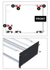
3. Slide an M3 bolt strip into each of the four mounting rails shown here.
