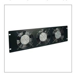
Tripp Lite's SRFAN3U SmartRack Panel-mount Triple Fan Accessory (for use with SmartRacks) is ideal for increasing the ventilation of SmartRacks, enclosures and server cabinets. The unit features (3) 4-in.-120V fans mounted in a 3U panel, 6-ft. (1.83 m) cord, and includes mounting hardware.
