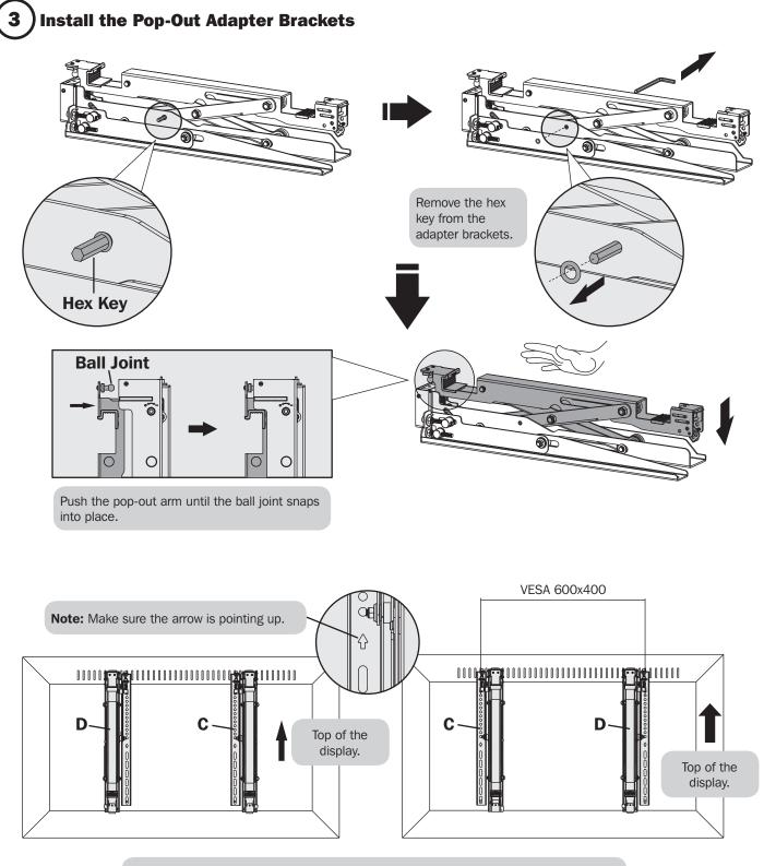
For VESA 600x400 mounting patterns, the "**D**" and "**C**" positions are flipped.
