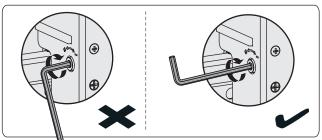
**Note:** Only use the long end of the hex key when tightening the adjustment screws.
