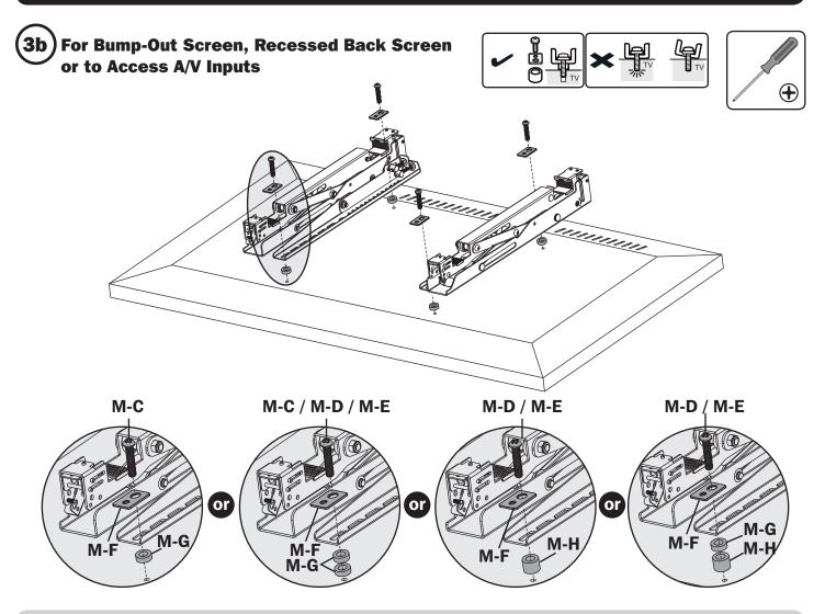
Note: Choose appropriate screws, washers and spacers (if necessary) according to the type of screen.
