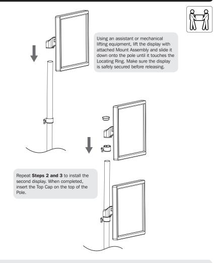
WARNING: Always ensure both monitors face forward. Turning the monitors to face backward may cause the unit to tip over.
