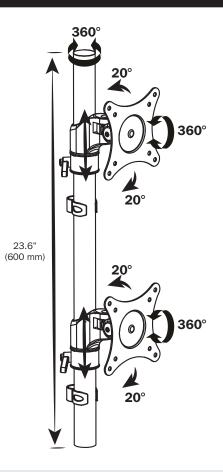
To adjust the desired location or tilt, use the appropriate Hex Key to adjust. Turn clockwise to tighten or counterclockwise to loosen.
