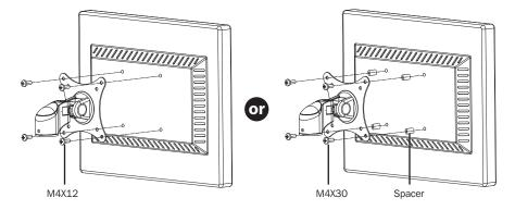
Lift the display and align the rear mounting holes with the mount assembly's VESA plate.
