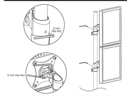
Use the appropriate Hex Keys to adjust the swivel. Turn clockwise to increase tension or counter-clockwise to reduce tension.
