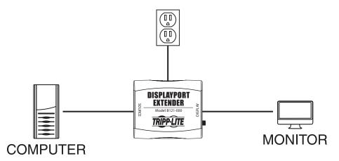
Connect the longer DisplayPort cable between the source and the *Source* port on the B121-000.
