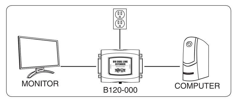
Connect the longer DVI-D Dual Link cable between the source and the connector on the B120-000 labeled "Source."
