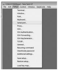
2 Select the COM port that is being used, and update the remaining settings as follows: Baud Rate (57600), Data (8 bit), Parity (none), Stop (1 bit), Flow Control (none).
