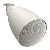
The PJ-304 is a projection speaker designed for ceiling and wall installations. Considered in architectural design, it can blend in with lighting equipment. The supplied swivel bracket allows for flexible speaker angle adjustment. The PJ-304 is driven on both high-impedance (100 V and 70 V) and low-impedance (8 #9b) lines. The input power (impedance) can be easily changed at the upper side of the speaker. The speaker is easy to repaint so as to meet a wide range of design needs.
