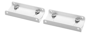
The HY-WM1W is used exclusively to mount the HX-5 series speaker system to a wall or ceiling. This bracket permits the speaker to be tilted downward up to 20° from the horizontal when the speaker is mounted on a wall, or tilted up to 20° from the vertical when the speaker is mounted on a ceiling. This bracket is designed for indoor use.
