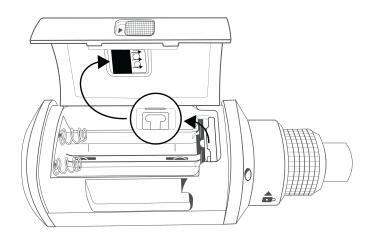
Note: If using AA batteries, set the battery type to ensure the transmitter's battery status indicator is accurate.
