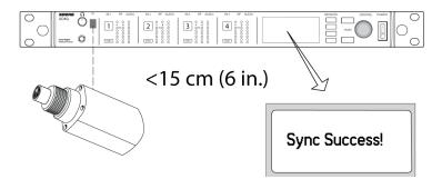
**Note:** Any change to the encryption status on the receiver (enabling/disabling encryption) requires a sync to send the settings to the transmitter. New encryption keys for the transmitter and receiver channel are generated on every IR sync, so to request a new key for a transmitter, perform an IR sync with the desired receiver channel.
