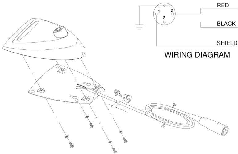
FIGURE 3: REMOVING THE BACKPLATE
