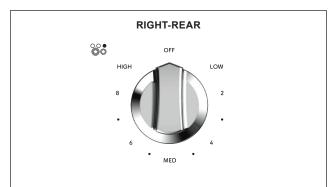
The RIGHT-REAR unit is controlled by the middle-right knob on the Control Panel, directly to the right of the touch screen.
