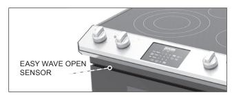
To use the Easy Wave Open feature, simply wave your hand in front of the sensor in two consecutive motions, either up and down or side to side.
