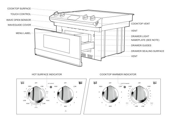
**NOTE:** Open the Microwave Drawer<sup>™</sup> fully. The label is beyond the back wall of the microwave cavity facing up from the flat surface.
