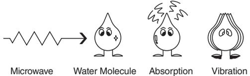
The microwaves cause the water molecules to vibrate which causes **FRICION**, i.e. **HEAT**. This heat then cooks the food. Microwaves are also attracted to fat and sugar particles, and foods high in these will cook more quickly. Microwaves can only penetrate to a depth of 1½ - 2 inches(4-5cm) and as heat spreads through the food by conduction, just as in a traditional oven, the food cooks from the outside inwards.
