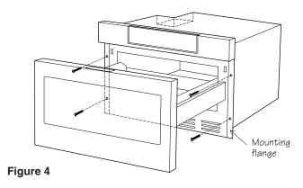
7. Secure the drawer with the 4 screws supplied.
