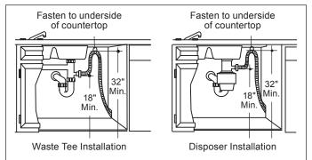
**IMPORTANT** When connecting drain line to disposer, make sure that the drain plug has been removed. DISHWASHER WILL NOT DRAIN IF PLUG IS LEFT IN PLACE.
