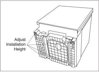
• Measure installation height and dishwasher height. Extend leveling legs out from the dishwasher base, 1/4" less than installation height.
