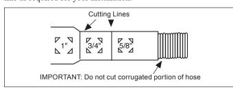
• If a longer drain hose is required, add up to 42" of length for a total of 10 feet to the factory installed hose. Use 5/8" or 7/8" inside diameter hose and a coupler to connect the two hose ends. Secure the connection with hose clamps.
