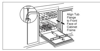
Fasten the dishwasher to the underside of the countertop with the 2 Phillips screws provided.
