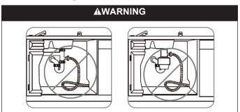
Do not connect the Drain Hose to the Sink Drain Waste Tee or Garbage Disposal without looping the Drain Hose underneath the sink with a High Drain Loop. Doing so will cause the Dishwasher to not drain properly, which may allow the drain water to back up in the Dishwasher tub or cause an "E1" error code.
