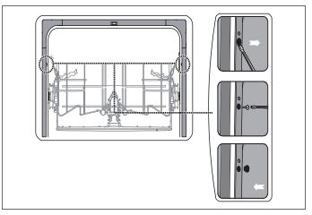
**IMPORTANT** Drive screws straight and flush. Protruding screw heads will scratch the top of the control panel and can interfere with the door's ability to close. If the gap is less than <sup>3</sup>/8" between control panel and the screws, method 2 is recommended.
