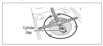
3 Empty the Cylinder filter and rinse it under running water.
