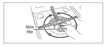
6 Inspect both the Fine filter and the Micro filter for debris and then clean them by holding the filters under slow running water.
