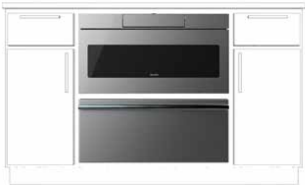
INSTALLATION WITH WARMING DRAWER BELOW
