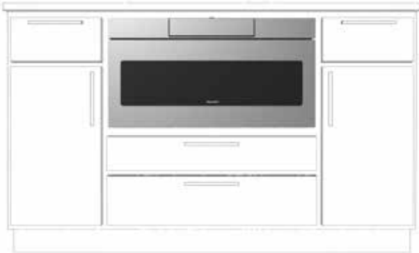
STANDARD INSTALLATION WITH DRAWERS BELOW
