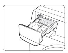
Add only liquid chlorine bleach to the **bleach compartment**. Do not exceed the **max line**.
