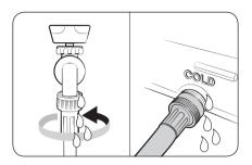
5. Open the water taps, and check for leaks.
