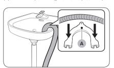
3. Route the drain hose to the drain system.
