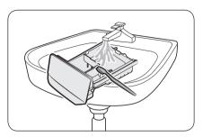
**4.** Clean the drawer components in running water using a soft brush.
