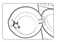
Remove the small circle of film (B) above the door latch before use.
