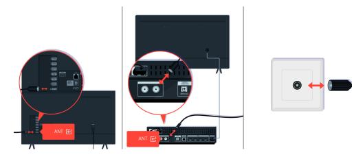
Check the antenna and input cable connections.
