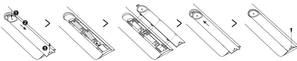
Match the polarity of the batteries to the symbols in the battery compartment.
