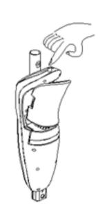
2. Open the water tank by unscrewing the water tank cap.
