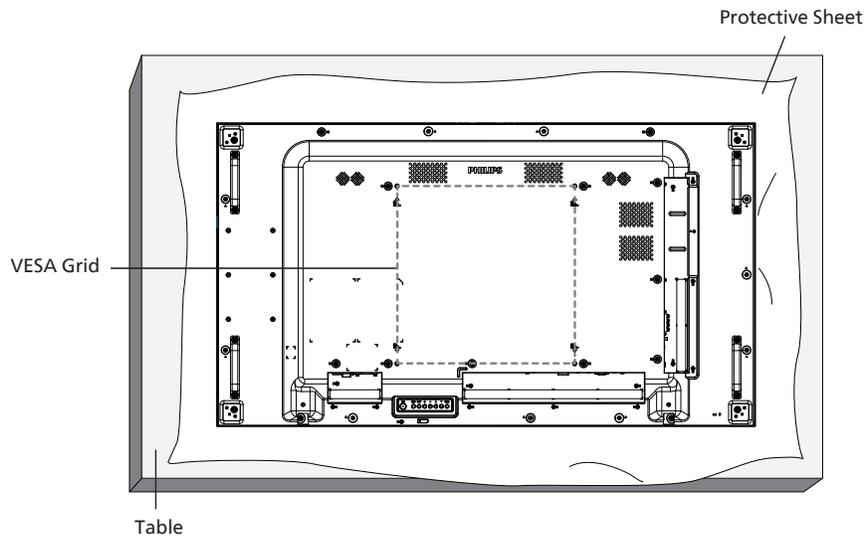
1. Spread a protective sheet which was wrapped around the display when it was packed on a flat surface. Lay the display face-down on the protective sheet to facilitate your operation without scratching the screen.
