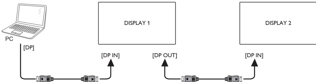
Connect laptop [DVI] to [DVI IN] of DISPLAY 1, connect the [DP OUT] connector of DISPLAY 1 to the [DP IN] connector of DISPLAY 2.
