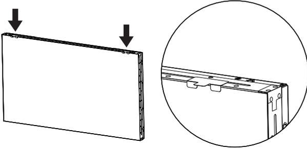
3. Install the top display carefully. After the displays are mounted, make sure you leave enough space between displays for removing the gap pad. If the pad is hard to release, adjust the position of the display to get enough space.
