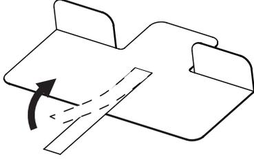
2. Stick the gap pad to the top surface of the display where another display will be stacked. Apply 2 gap pads on the top surface.
