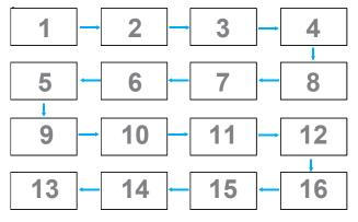
**Note:** To use this function, serially connect all machines with RS-232 cable and set their Network control port to RS-232
