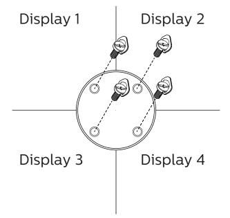
• Use the "Edge Alignment Kit-2" for two adjacent displays.
