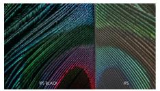
A newly developed technology, IPS Black offers the same 178/178-degree viewing angles but with an improved color contrast ratio that is essential for a multi-monitor setup. In addition, it is well suited for professions that demand color accuracy by expressing deeper blacks and better color in 4K clarity; thereby making colors more vivid.
