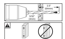
ENG Mounting hole must center on stud.
