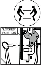
OPTIONAL: Insert M5 x 10mm type-F socket pin screws to lock latches.
