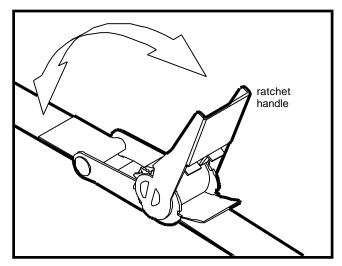
To release, compress release bar and open ratchet handle 180°.
