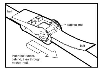
Pump ratchet handle to tighten belt. For secure hold, ratchet reel must have at least two layers of belt around it.
