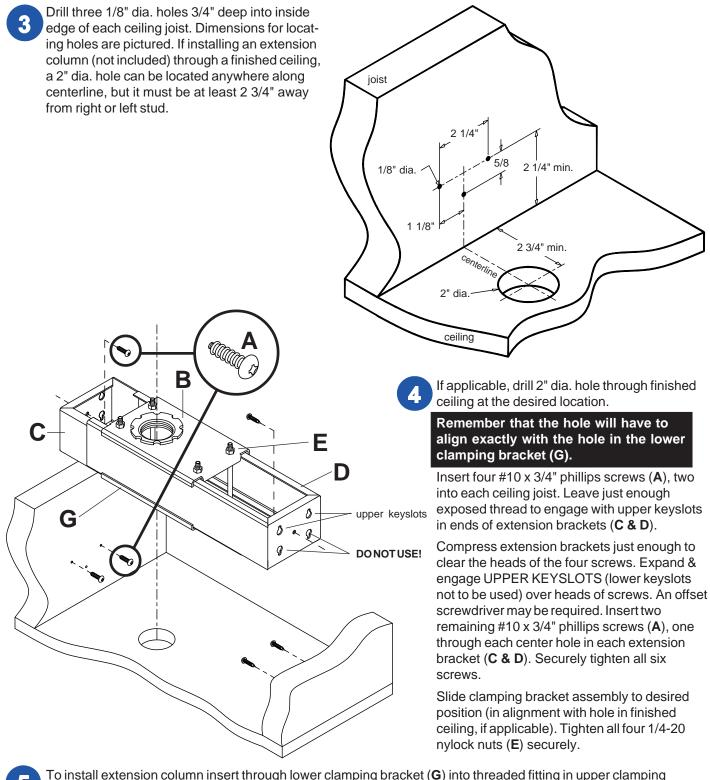
To install extension column insert through lower clamping bracket (**G**) into threaded fitting in upper clamping bracket (**B**). Tighten four or five complete turns until securely tight.
