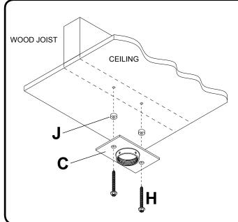
For Optional Cord Management, install two spacers (J) between ceiling plate (C) and ceiling.
