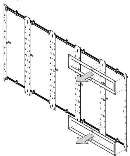
ENG Optional: For shallow depth installations, flip wall bracket orientation as shown. 2.25" (57mm) 2.60" (66mm) MIN MIN display tile display tile wall 0 0 2.65" (67mm) 3.05" (77mm) MAX MAX
