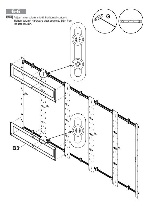
ENG Continue adjusting inner columns to fit horizontal spacers until all are level. Tighen column hardware after spacing
