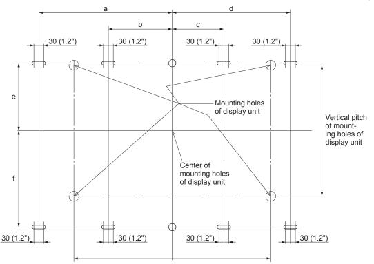
Horizontal pitch of mounting holes of display unit
