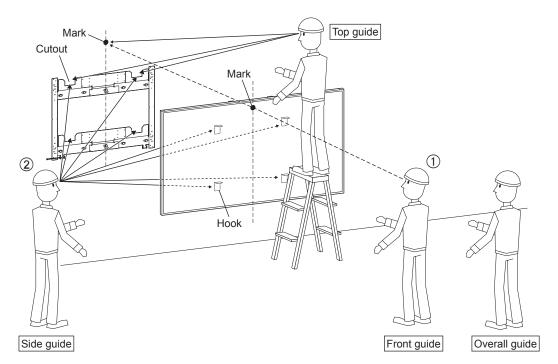
• When attaching the set mounts to the bracket on the wall surface, attach it while pressing the entire display unit onto the wall.
