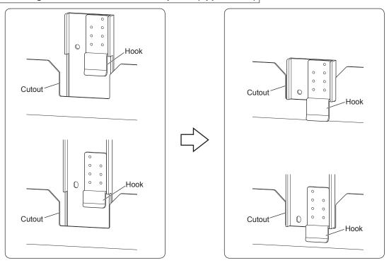
• As shown in the following figure, visibility is limited when viewing from the side so checking the positions of the cutouts and hooks will be difficult.
