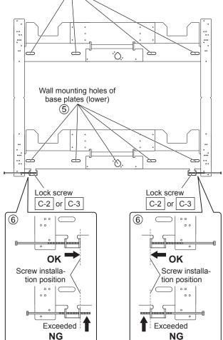
Install the lock screw on either the left or the right.
