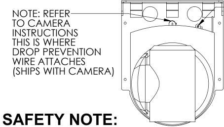
INSTALL 3MM SCREW FLAT & LOCK WASHER TO SECURE CAMERA TO MOUNTING **BRACKET** (THIS HARDWARE SHIPS WITH CAMERA)
